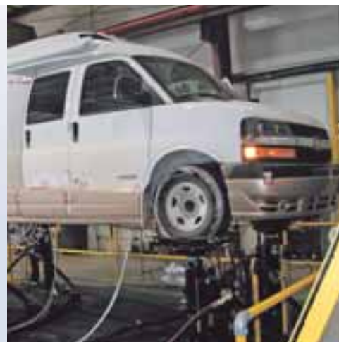
“Automotive manufacturer” style durability testing allowed us to quickly identify and implement numerous design improvements which would otherwise only become apparent during the normal life of the first ones of each new model built and sold.
