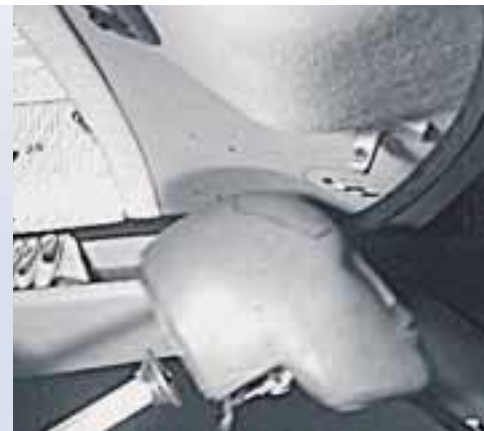
Occupant head protection testing is intended to ensure occupants have additional head protection from interior components during crashes.
