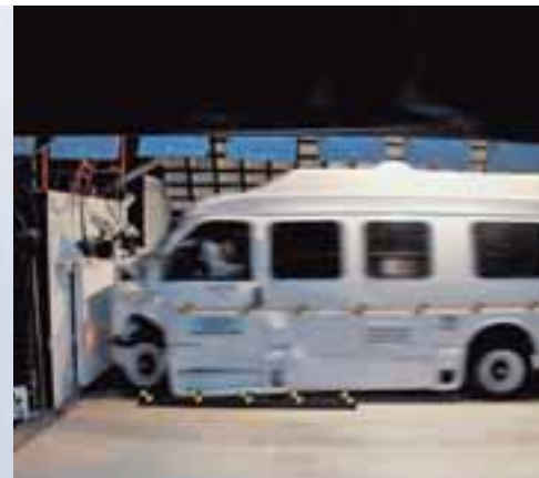
For frontal impact testing, the test vehicle impacted a fixed barrier at 30-mph (48 km/h). Again our test vehicle did not leak any fuel.
