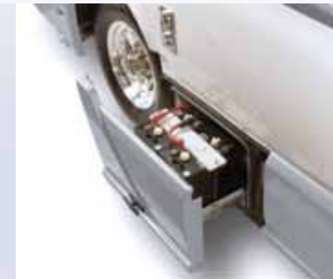
190-Popular, 210-Popular and Sprinter based models feature two auxiliary deep cycle 6V AGM batteries with 220 total amp hours. On 190 and 210 models they're located on a convenient slide-out tray.
