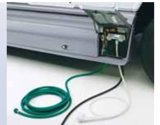
There is a separate compartment for the city water connection with quick disconnect and detachable power cord for trips away from the campsite. An exterior shower is located here as well.
