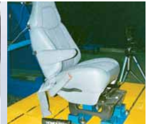
Seating system testing minimizes the possibility of failure of the seats, their attachments and their installation.
