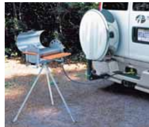
External propane barbecue connection with quick disconnect (all models except 190-Simplicity and 210-Simplicity).
