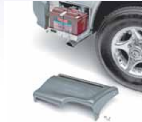
On the 170-Versatile (shown), 190-Simplicity and 210-Simplicity, a large capacity auxiliary 12V AGM battery is totally concealed yet easily accessible on slide-out tray.
